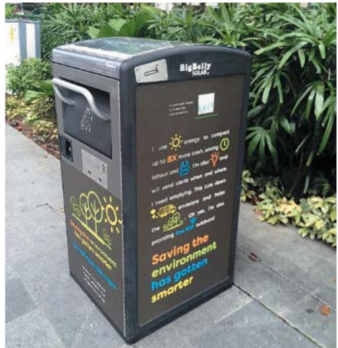
One of the solar powered BigBelly bins along Orchard Road which comes with an automatic compacting function and WiFi
