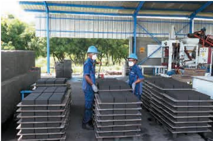
*Paving blocks made from waste fly ash and bottom ash from the power plant*
